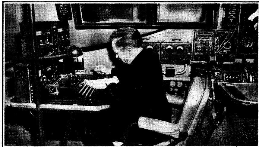
THE RADIO OFFICER at his post in the radio control room on the upper deck of Pan-American Airways Yankee Clipper, which inaugurated the new transatlantic air service. A hundred watt transmitter, WCBN, which was installed by the Columbia Broadcasting System for the transmission of commentaries during the initial flight, is located in the lower compartment of the plane's nose.
